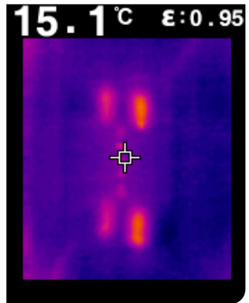
*The FLIR TG165 proved to Recochem that thermal imaging cameras can see through cardboard and check the pattern and size of the applied glue spots. This meant that it was no longer necessary to destroy the boxes for inspection.*
