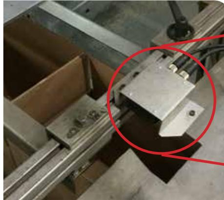
The AX8 camera is set up to look at predefined areas of the flaps where glue should be applied, and verify spot sizes and their temperatures.
